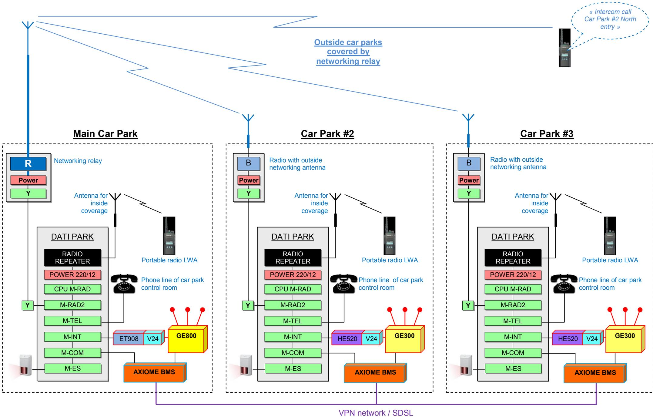
The radio system is built with HFI Din modular hardware:
